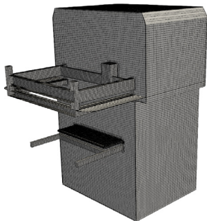
Fig. 1: Finite element mesh of the 3D printer used in OpenFoam CFD simulations.
