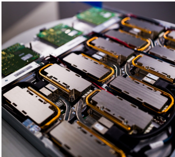
Fig. 1: HPC Vega CPU blade - 3 CPU nodes Fig. 2: HPC Vega GPU Partition usage in 2022 - month-by-month
