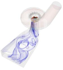
One of the successful outcomes of the CFD training is demonstrated, for example, by the simulation of partial load behaviour of a Kaplan turbine.
